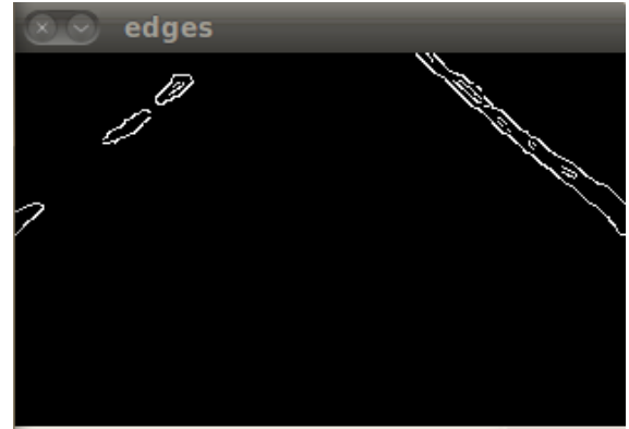
Figure 13. Image after Canny edge detection
