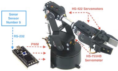
Figure 14. Connection between the mbed and the mechanical arm
