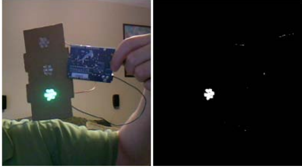
Figure 7. HSV filter of the green traffic light
