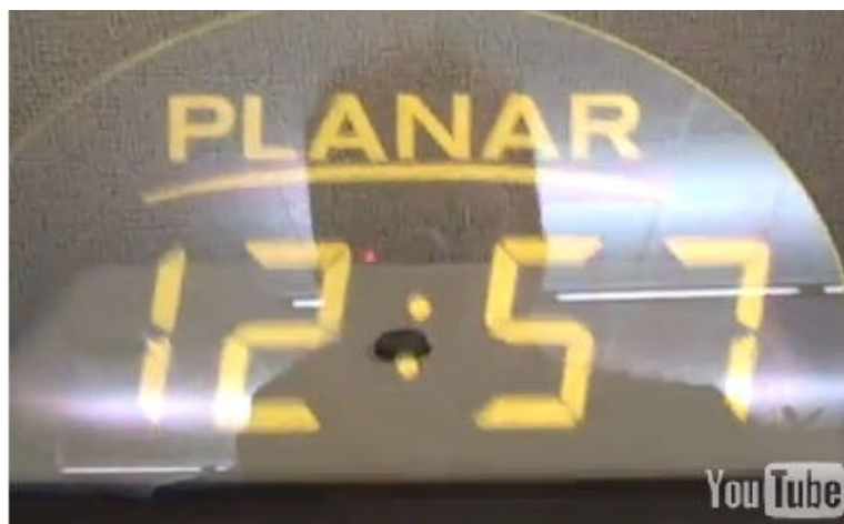
Figure 3: Planar's transparent electroluminescent (EL) display 6
