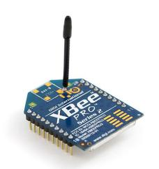
potentially transmit wireless signals around the world and beyond.<sup>2</sup> For our simple demonstration of a wireless communications link, we propose to take two Xbee (hardware IC chip shown below) Pro 50mW wireless modules and create a Zigbee (protocol) wireless link between a PC and a sensor.
